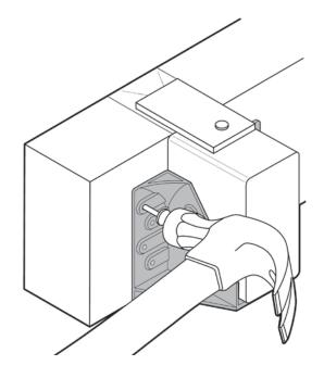
Once both top left and right hand connector nails are in place remove the "Jig" and insert the remaining nails to attach the hanger to the bearer –
